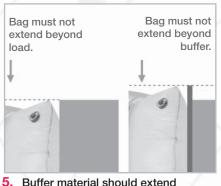
Buffer material should extend slightly beyond the load.
