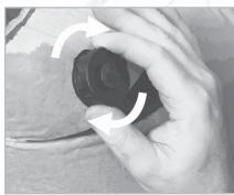
Remove the inflator and attach the valve cap. Ensure that the cap is tightly secured.
