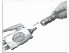
2. Put the connector of the air tool into the quick coupling. Press them firmly together.
