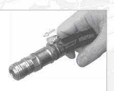
3. Move the clamp over the tube and the pillar of the coupling.
