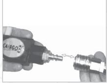
2. Put one of the valve connectors into the quick coupling of the air tool.
