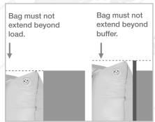
Buffer material should extend slightly beyond the load.
