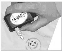
Unlock the MouseTip by pushing the slide pin fully to the left position.
