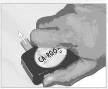
Lock the MouseTip by pushing the slide pin fully to the right position.
