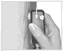
Install the MouseTip and slide the MouseTip over the valve.
